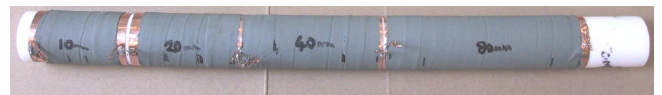
Figure 5. A PTFE tube with four sample-lengths of the stress-grading tape between electrode pairs.
