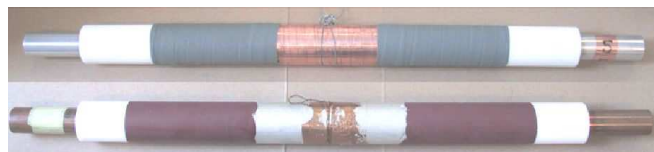
Figure 1. Pictures of simple stress-graded model bars using B-stage tape (top) or corona-protection paint (bottom). The total length is about 0.5 m.
